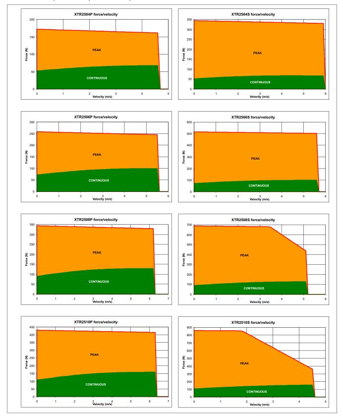
Figure C.5 - XTR25 force / velocity profiles
