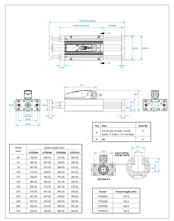
Figure 2.1 - XTR25 Outline drawings and mounting details
